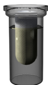
Stage 1 - Boiling Boiling solvent is covering the sample so that extractable material can be liberated.
