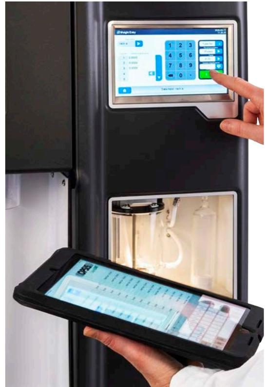
TRANSFER UTILITY ON IPAD TO TRANSFER WEIGHTS TO THE KJELROC ANALYZER
